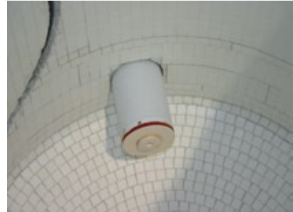
Grinding chamber with ceramic lining
