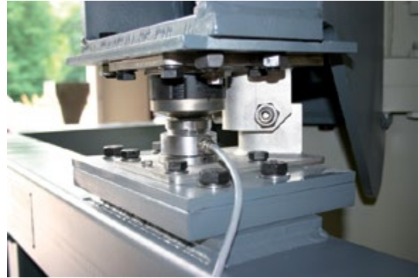
Load cell, mounted on CGS
