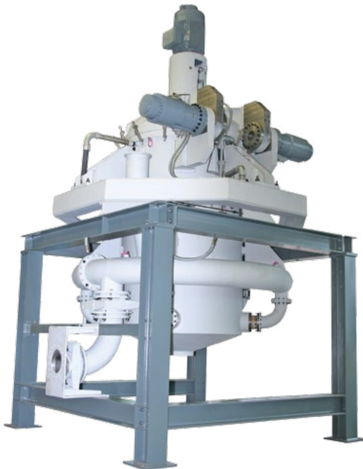
Fluidized Bed Jet Mill Type CGS 180 for milling air consumption of 11 660 m 3 /h.
